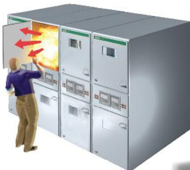
Typical switchgear without PACS Plenum System
